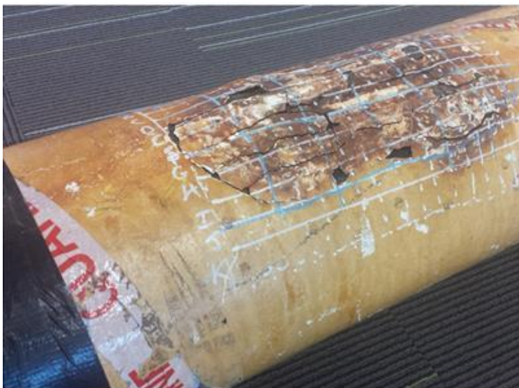
PEC scan from outside—Compensated WT C-scan
